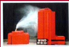
Figure 1b. Plume impact on taller upwind building.
