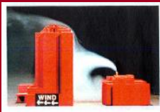
Figure 1a. Plume impact on taller downwind building.
